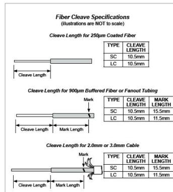
\*Alternative cleavers were also tested. Those with a guaranteed maximum 1° cleave angle for single-mode fibers and a maximum 2° cleave angle for multimode fibers provided acceptable results.
